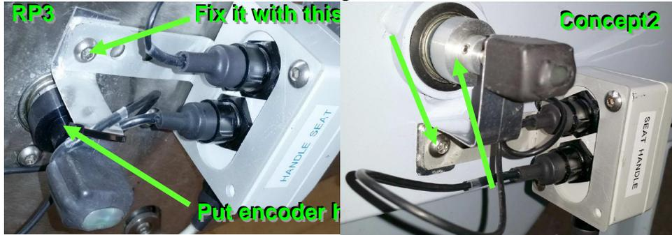
To adjust the position of the hub, release two grab screws and slide the hub of the encoder shaft to make full contact with the nut on the erg. You can tighten two grab screws to fix the hub on the nut, but it may work better, with less oscillations, without fixing it.
