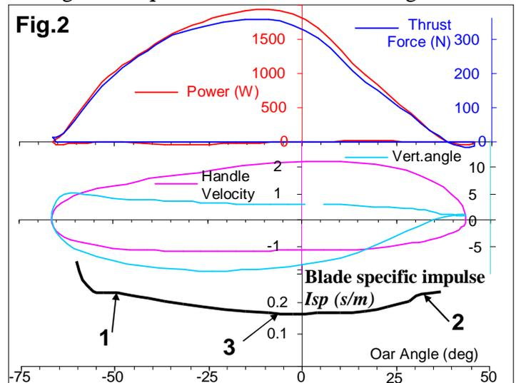
The blade specific impulse  $I_{sp}$  looks quite even during the drive. Its higher value ~0.23 s/m was found at the beginning and the end of the drive (1, 2); the lowest 0.16 s/m - at the perpendicular position of the oar (3). The average  $I_{sp}$  of underwater blade work was 0.19 s/m at this sample. It decreases at higher stroke rates and boat speeds from 0.27 at rate 20 down to 0.17 s/m at 41 str/min.
