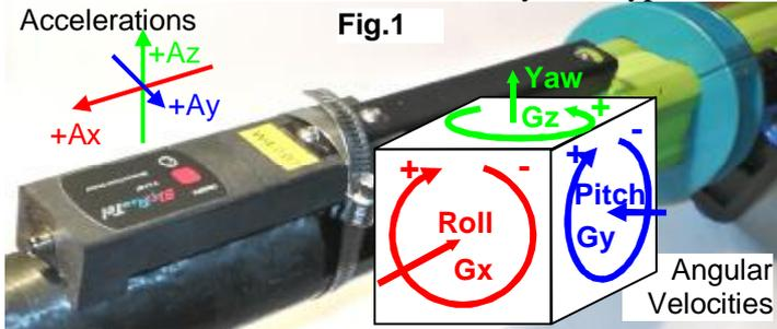
The frame of reference was set similarly to the boat motions analysis (RBN 2012/03) and the axes directions were defined by the design of the sensor. Fig.2 shows the oar accelerations and angular velocities together with the handle force and oar vertical angle obtained from the right oar in M1x at 30 str/min:
