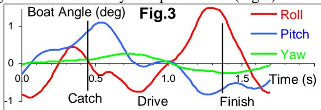
Though these angles are not strictly connected to the reference frame of the Earth/water, they are useful for evaluation of relative rotational motions of the boat and could be interpreted in the following way:
