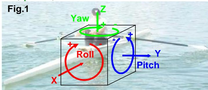
BioRowTel measurement system (1) is equipped with 3D gyroscope, which allows measurement of angular velocities of the boat rotation around all three axes. The agreement on the directions was made:
