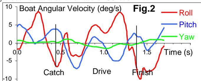
Angular velocities are difficult to interpret and make meaningful for a coach and rower. They were integrated into angles of roll, pitch and yaw, and then offsets were added to each of them to make the average over the stroke cycle equal to zero (Fig.3).
