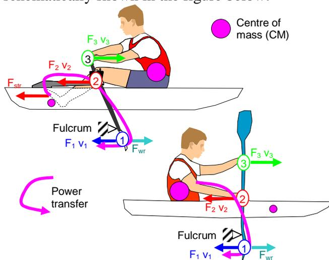
In both cases, the oar works as a lever of the second order with the fulcrum somewhere close to the blade. It is not easy to determine the exact position of this fulcrum, owing to slippage of blade in the water. If we consider forces, then there are three points of force application at the oar:
