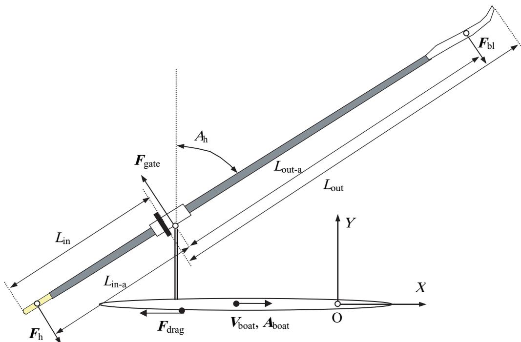
Fig. 1 Coordinate system and forces acting on the boat and oar
