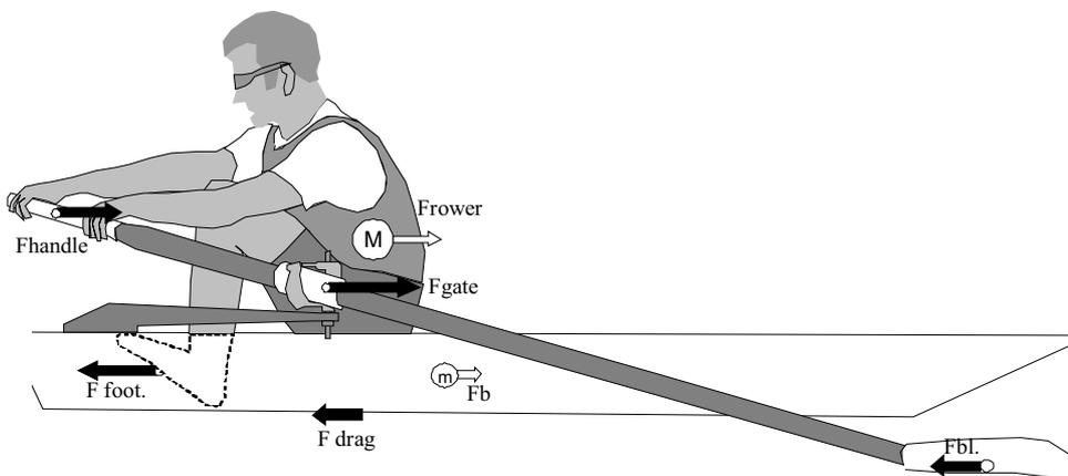
Fig. 10 The main forces in the rower–boat–oar system
