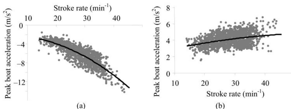
Fig. 3 Dependences of (a) the negative peak of the boat acceleration at catch and (b) the first positive peak of the boat acceleration during the drive (b) on the stroke rate
