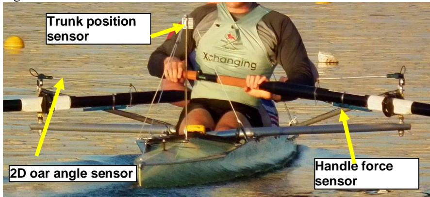
Two-dimensional (2D) oar angle sensor measures position of the oar shaft in horizontal and vertical planes. This allows to define the track of the blade relative to water level and hence catch and release slips and effective angles.
